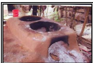
Two potholes stove
