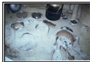
Three pothole stove in Dang
