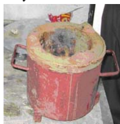
Metal stove with clay lining
