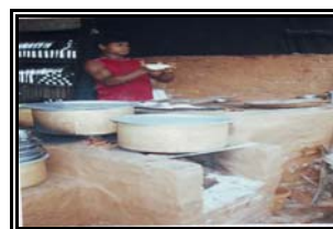
Two potholes and tandori stove
