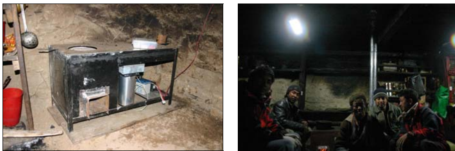
Photograph 11: Ujjeli Chulo with TEG (left) and room after installation of Ujjeli Chulo (right)
